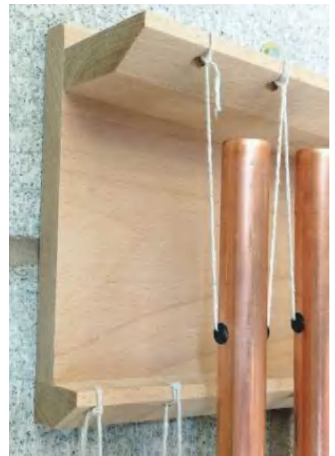
PIC 2. Tubes cut, drilled and fitted with grommets. It then occurred to me that for playability, the 'black notes' had to be positioned within reach of the 'white notes' just as they are on a piano. This gave rise to a sloping top rack. I had initially thought of making the set floor standing but that would have been a large construction and unwieldy if it were to be moved around. Rather, I made my bracket to screw to the wall
